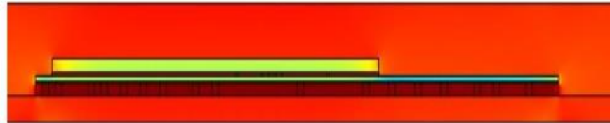
Warpage-induced stress distribution
